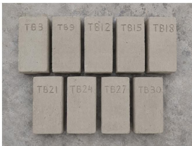
Figure 1. General appearance of bentonite-based brick specimens dried under natural conditions
