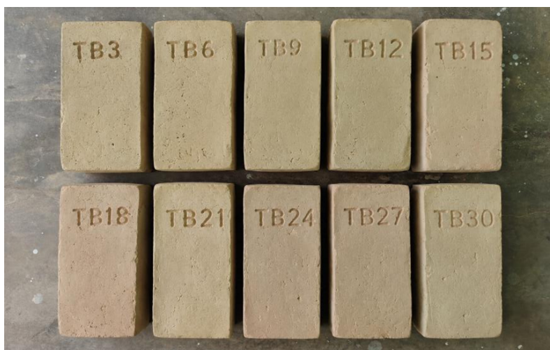
Figure 2. General appearance of the fired brick specimens
